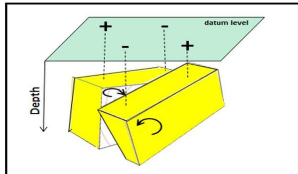
Figure 7. Example of rotated block along vertical faults
